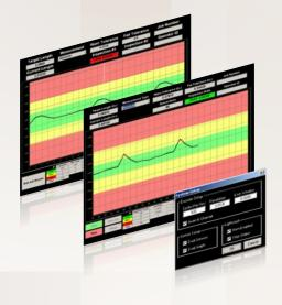
SETUP: A easy-to-use setup screen allows the operator to program details about each job, or load information from a previous run.
